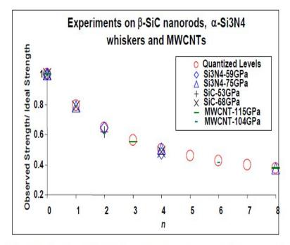
Quantized strength levels: experiments on β-SiC nanorods, α-Si<sub>3</sub>N<sub>4</sub> whiskers and MWCNTs, and QFM predicted values.
