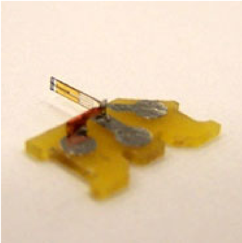
Quartz Tuning Forks, typically f=32\text{KHz}
