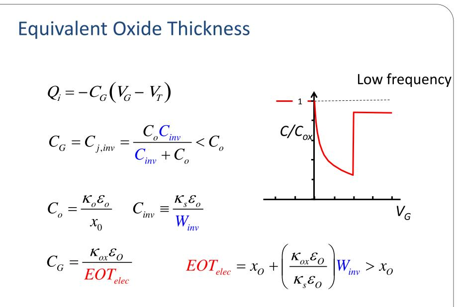
'Equivalent oxide thickness - electrical '
