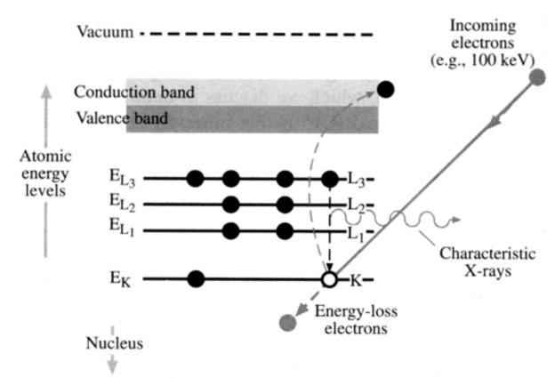
High energy electron scatters inner shell electron ( $E > E_c$ )
