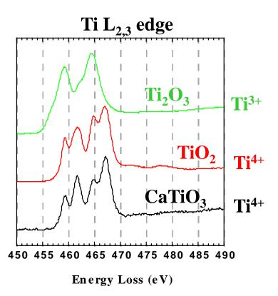
Ti  $L_{2,3}$  edge from trivalent  $Ti_2O_3$  differs markedly from tetravalent compounds  $TiO_2$  and  $CaTiO_3$ .
