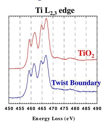
Ti  $L_{2,3}$  edge from twist boundary closely matches edge structure of  $TiO_2$  standard ( $Ti^{4+}$ ).
