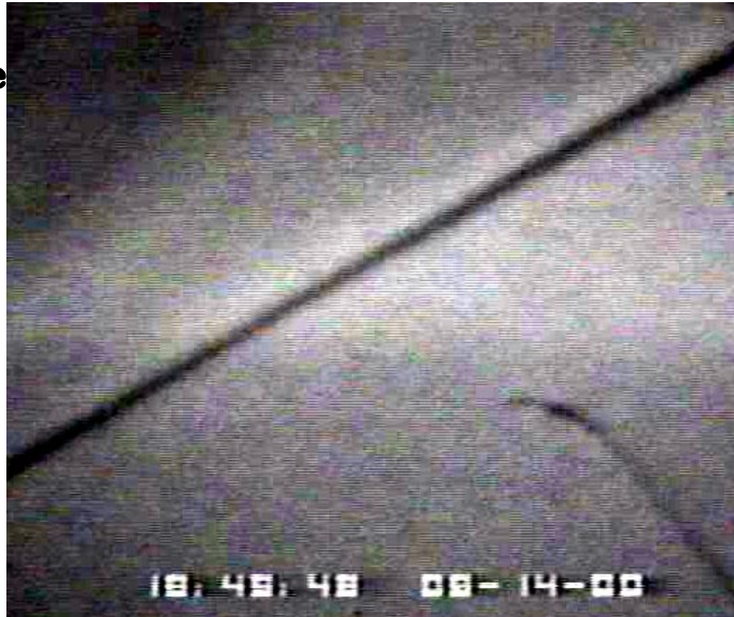
Interaction between threading and misfit dislocations in a SiGe heterostructure
