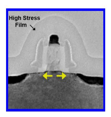
Highly tensile silicon nitride capping film
