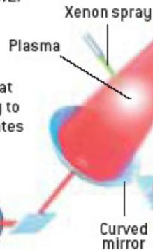
2 Curved and rectangular multilayer mirrors focus a selected wavelength and direct it toward the mask
