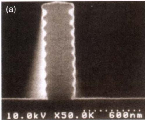
Interference between incident and reflected photon beams can lead to a standing wave pattern in the resist.
