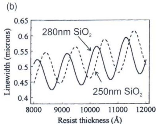
Reflections can also occur at buried interfaces, thus leading to a dependence of linewidth on buried layer thicknesses.
