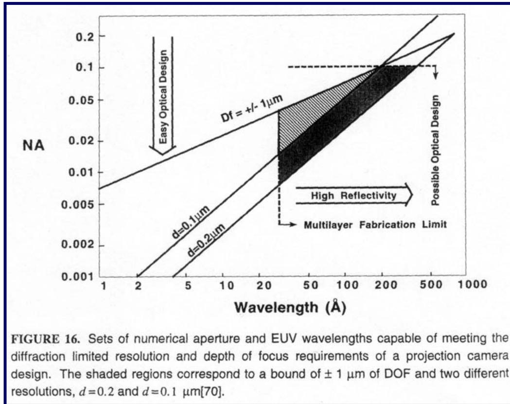
FIGURE 16. Sets of numerical aperture and EUV wavelengths capable of meeting the diffraction limited resolution and depth of focus requirements of a projection camera design. The shaded regions correspond to a bound of  $\pm 1 \mu\text{m}$  of DOF and two different resolutions,  $d=0.2$  and  $d=0.1 \mu\text{m}$ [70].
