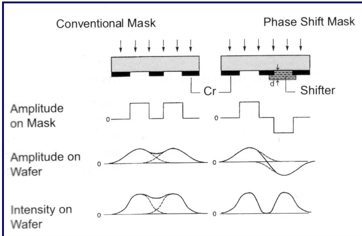
→ Minimizes diffraction effects but complicates mask making
