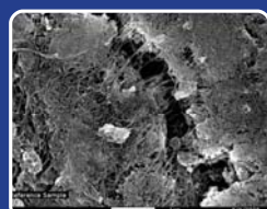
SEM secondary electron images of CNT reference sample (JEOL JSM-7300 FE-SEM)
